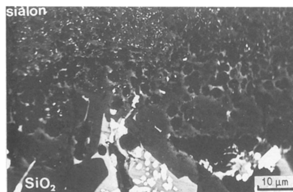
Figure 3 An enlargement of the reaction zone closest to the sialon in the \text{Cu}_2\text{O} -sialon system. The micrograph shows the occurrence of cavities in the \text{SiO}_2 matrix.
